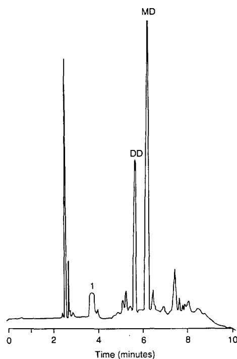
Fig. 3. CZE electropherogram of a solution of IFM and DDTC after derivatisation at 50°C for 40 min. MD=mono-derivative of IFM, DD=di-derivative of IFM, 1=elution time of neutral species.
